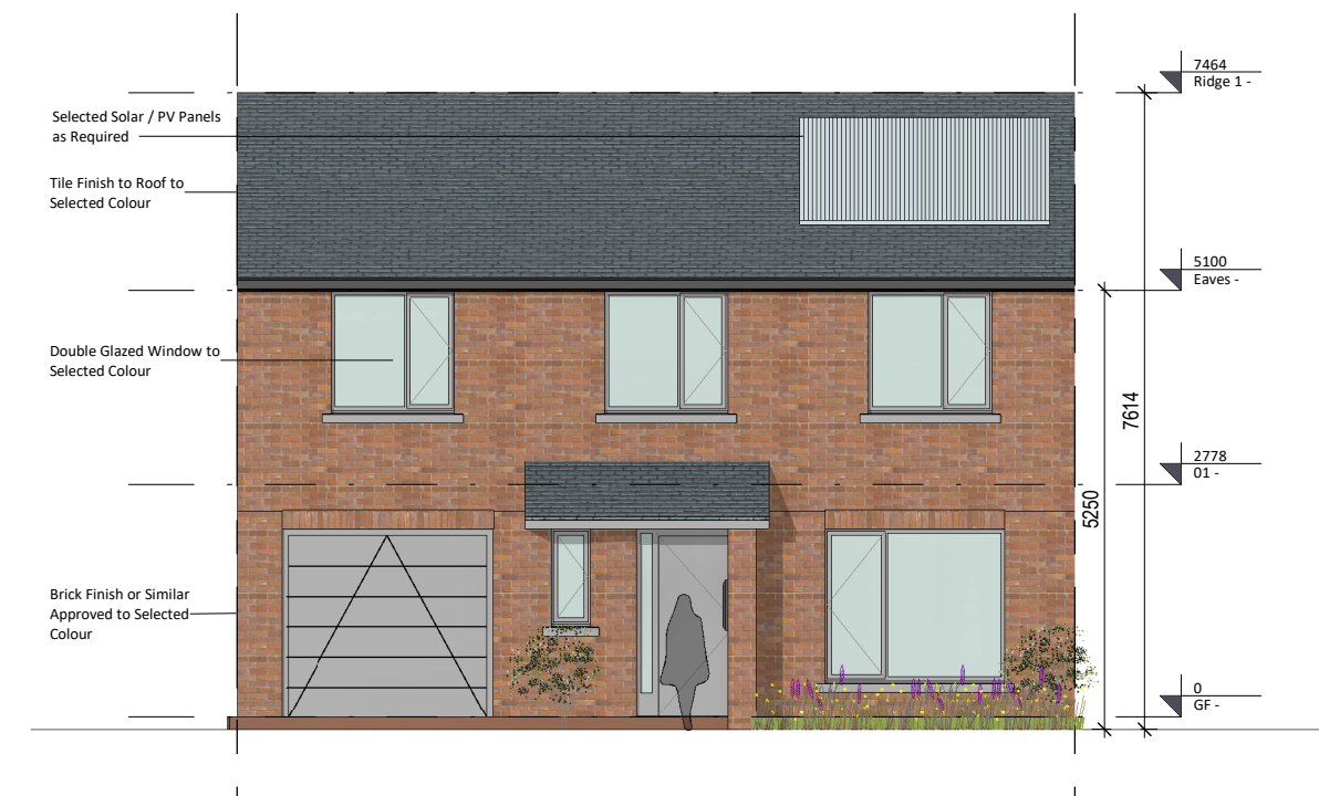
⑥ Front Elevation Type A ( Full Brick) 1 : 100
